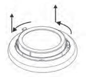
Hold the rotating housing on the activation hook, turn the glass retaining ring with glass to the left.
