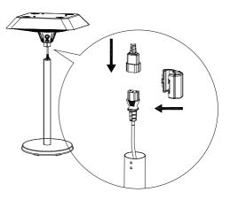
4. Push the Heater Head onto the pole and fix in position using the 3x8mm screws.
