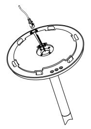
3. Connect the power cord plug to the socket in the heater head.
