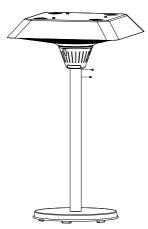
5. Fix the power cord with the press clips in the base.
