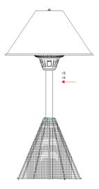
6. Pull the power cord gently out of the base as much as possible. Fix the power cord under the weighted base using the supplied 4pcs M4 nuts.
