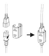
5. Push the heater head on to the tube and fix it in position using the supplied 2 x M4\*8 screws.
