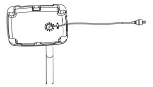
6. Fix 2pcs fixing part on the base with 4pcs M6\*10mm screws, then Fix the heater on the floor. Bore two holes in the floor, fix the heater by two expanding bolts on the floor.
