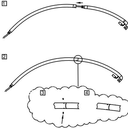
2. Connect the curved pole assembled in the previous step to the straight pole (as pictured). Insert 3 x M6X8 screws into the corresponding holes and tighten until secure.
