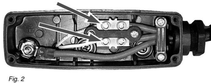
4. Disconnect the emitter from the connector blocks by unscrewing the screws highlighted above in Fig. 2.
