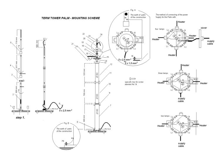
Put the cast iron base on a horizontal plane.
